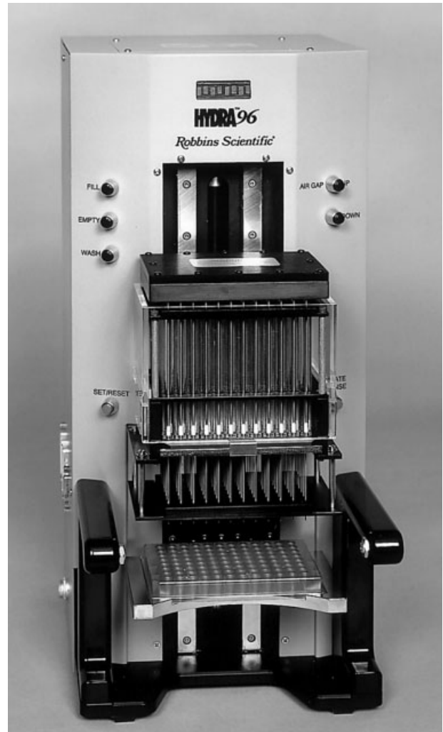
FIG. 1. Hydra 96 microdispenser used for automation of various steps in the flow-FISH protocol (high resolution image kindly provided by Robbins Scientific, Sunnyvale, CA).
